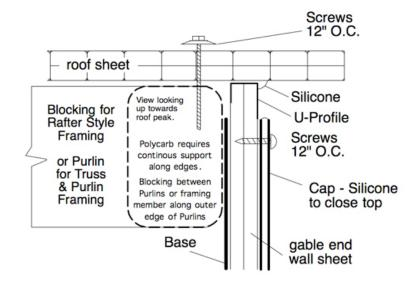
**Note:** Adjust position of last rafter (or vertical blocking between purlins and framing member) to accommodate overhang and to provide a continuous member to attach polycarbonate sheet to.
