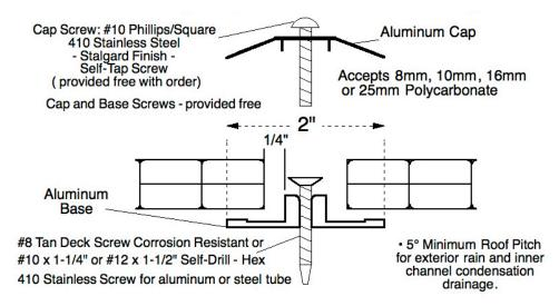
**Note:** Install base straight or alignment issues may occur when attaching cap. Check with local building codes for recommended purlin/girt spacing to support snow and/or wind structural loads for your area.
