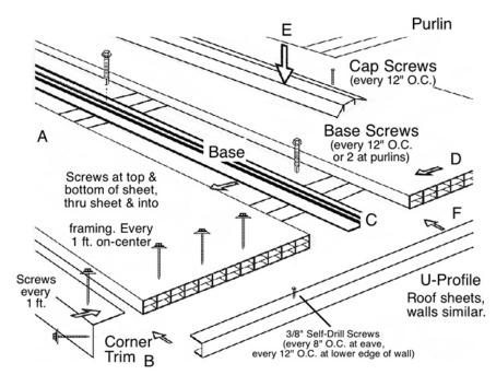
**Note:** Always pre-drill holes in Base and Cap for screw placement. Self-drilling screws are 'never' meant to drill through these components. Self-drill screws pass through components, fastening both to the frame.
