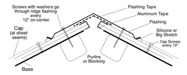
**Note:** Butt cap to flashing and seal. If using rafters, drawing shows blocking. For applications in high wind areas or expansion and contraction is a concern, use Big Stretch caulk.
