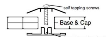
Trilobular Screws: #2 Phillips-Sq. Combo. Round tip for swift threading into screw race. Hurricane Strong!
