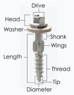
Fasteners should penetrate the roof or wall of the structure by at least one (1) inch. At least a 14mm (.551") neoprene bonded washer is recommended for most applications. If aesthetic concerns arise, a smaller washer may be used if it provides a flat bearing surface and creates an effective seal.
