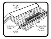
Always check the corrugated sheets and closure strips for proper fit. Closures may come with adhesive, should match sheet profile, and must be compatible with polycarbonate.
