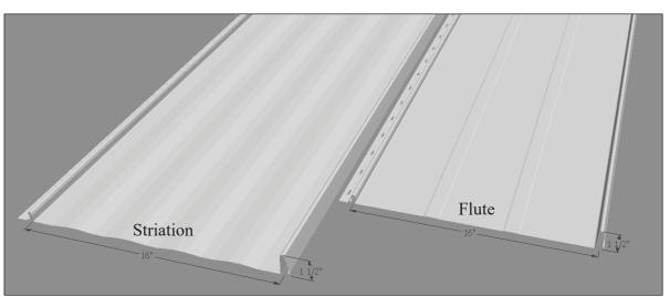
In addition to its unique and attractive look, Snap-Lock Standing Seam Metal Roofing has hidden fasteners that help eliminate the chance of roof leaks. The Standing Seam panels have a tall 1.5 inch rib height and are available 16 inch wide panels with 2 different profiles; Striation Rib or Fluted Rib. Snap-Lock Standing Seam is made out of a sturdy and durable **26 gauge** metal.
