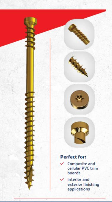
Our self-tapping Re-Fine Screw<sup>™</sup> is a cousin of the Fine Screw. With a double twist at the head for drawing strength, the Re-Fine Screw is ideal for siding, railing spindles, PVC and small adjustments. Available in U-Gold or White coating.
